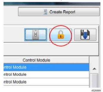
**Note:** The LOCK PARAMETER BUTTONS must be selected after each parameter has been selected to be graphed.
