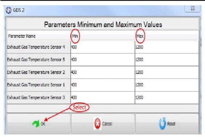
**Note:** When selecting the temperature values, the parameters should be all on the same scale.
