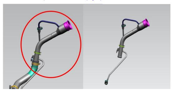
Fig. 1 Upper Fuel Fill Tube
