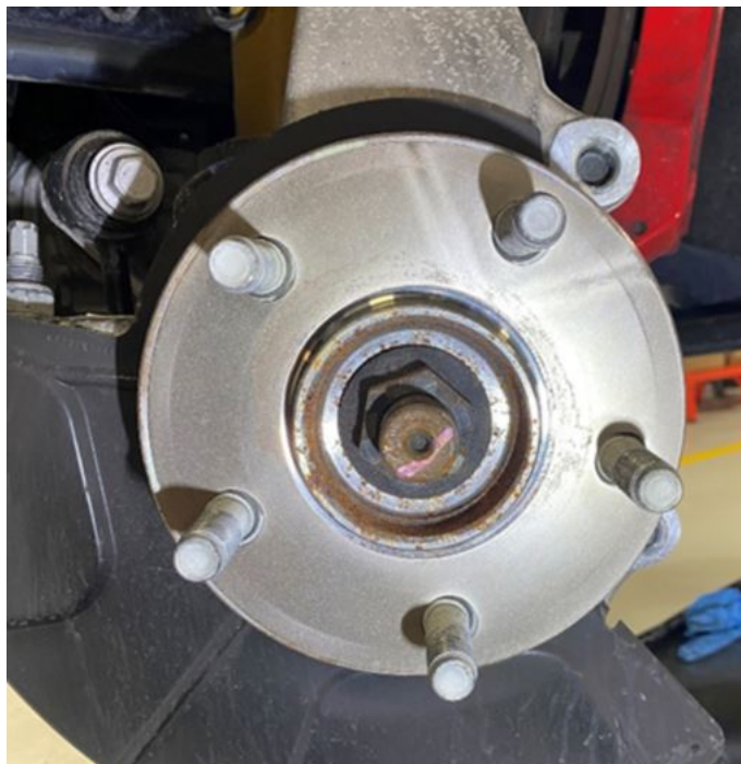
Fig. 3 Friction Disc Installed On Hub
