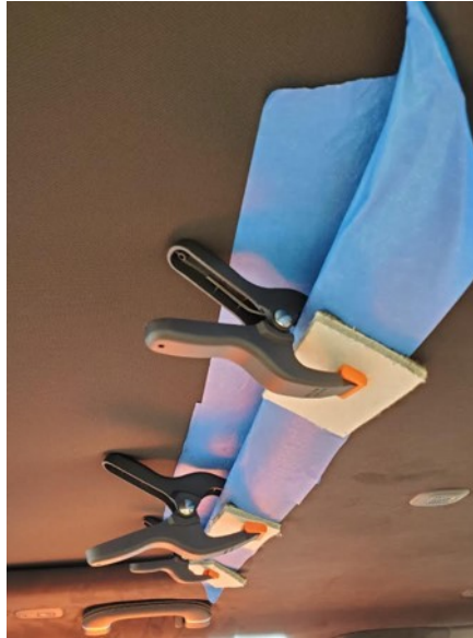
Fig. 5 Rear Area Clamped
