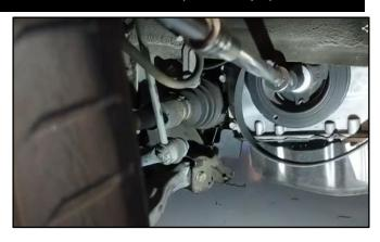
6. Show the engine being cranked and torque specification exceeding 94 lb.ft. torque.
