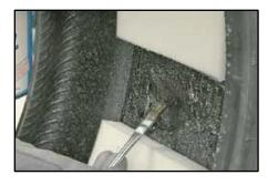
7. Install the plug patch until firmly flat inside the tire and roll out patch surface to promote adhesion.
