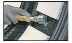
8. Cut off any excess plug on the outside of tire so that it is even to tread surface.
