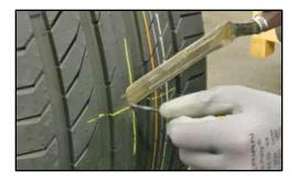
9. Apply tire cement glue over the patch surface area where foam patch was cut out and removed.
