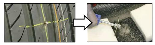
6. Apply cement glue to the tire puncture area and plug patch.
