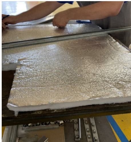
Figure.4. The cutting operation of sponge basotec
