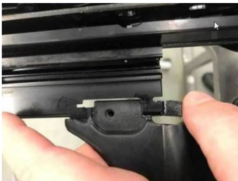
Figure 7. Areas to clean using cleaning solution D 009 401 04.
