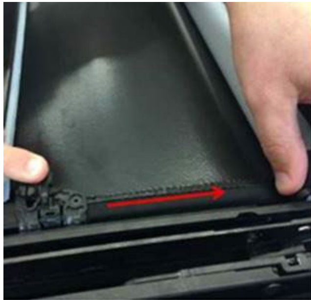
Figure 4. Push the material back to expose the bolts.
