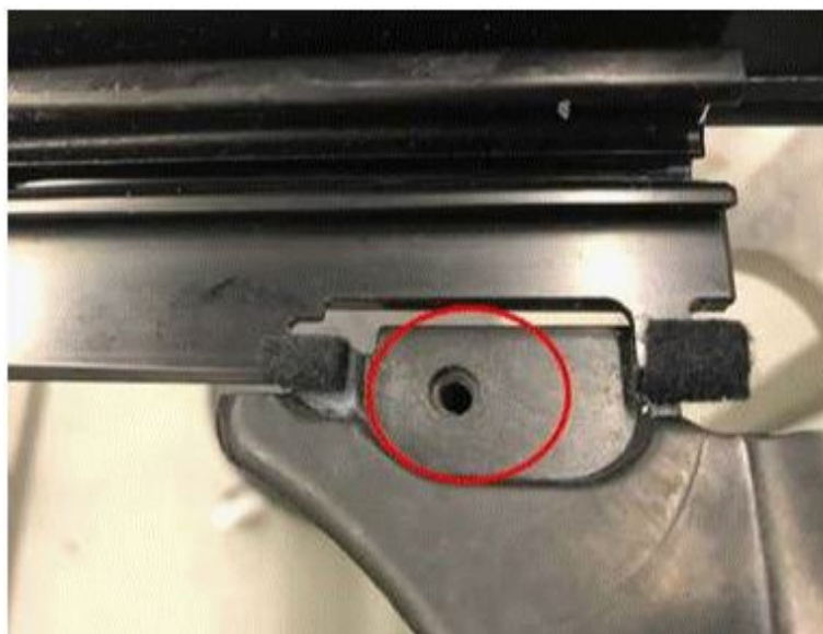
Figure 10. Apply thread locker in this area.
