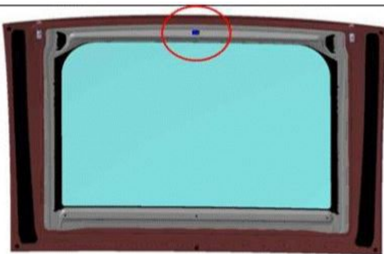
Figure 17. Area of sunroof glass panel structure to be prepared.
