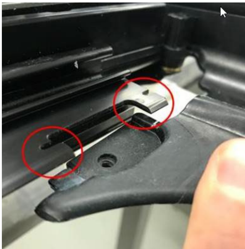
Figure 7. Areas to clean using cleaning solution D 009 401 04.
