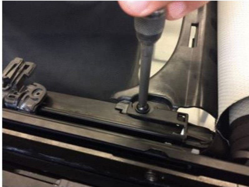
Figure 11. Torque screws to 3Nm.
