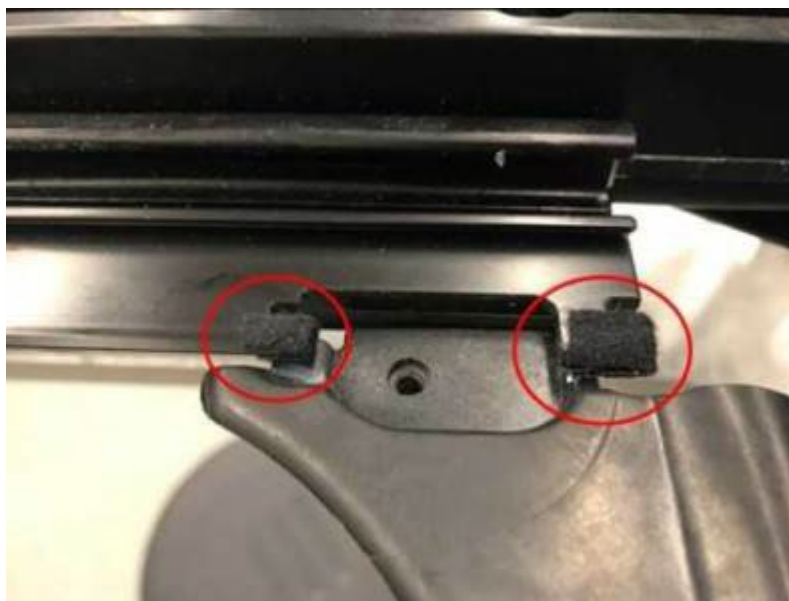
Figure 9. Apply felt tape on points shown. The tops and bottoms of the tabs must be isolated.
