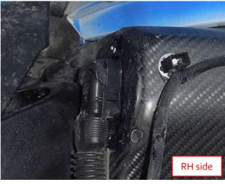
13. Refit the RH front wheel arch rear guard:
