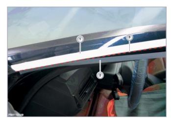
This will provide a reference point just below the masking tape to install sliding tape in step 4
