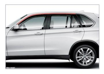
2. Clean the upper door jamb in the area shown (on the body) using silicone remover concentrate 83 12 5 A16 119 of the affected door.
