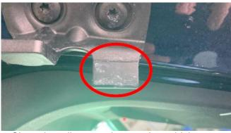
2. Apply Berucoat AK 978 P/N: 83 19 2 358 109 anti-squeak paint to the wedging element. Allow the anti-squeak paint to dry for 8 minutes with the tailgate open.
