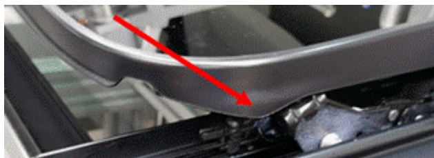
Figure 1. The front sunroof glass panel side skirt is deformed due to a protruding water guidance washer.
