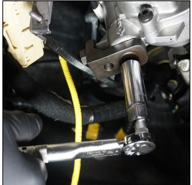
19. Remove the tool from the MDPS housing and inspect the bearing.
