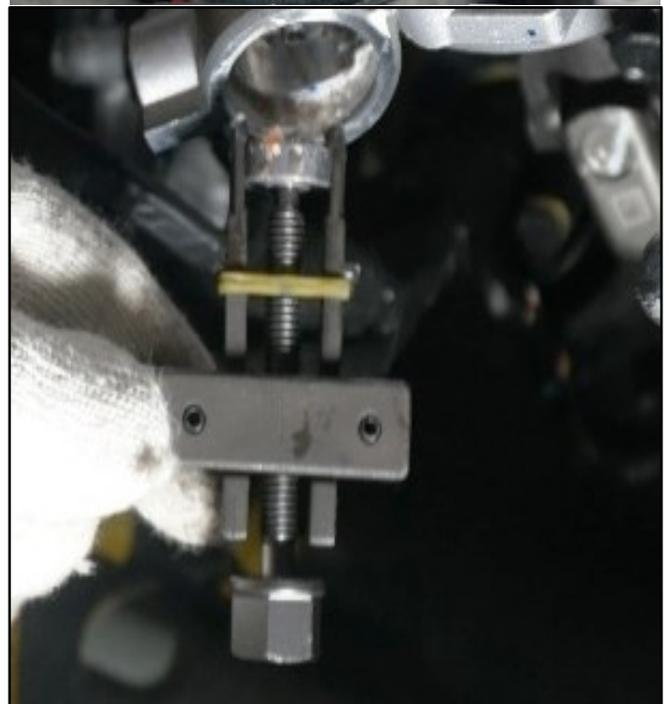
14. Use the supplied paper stick to remove the excess grease.
