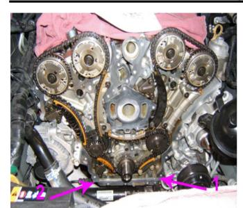
9. Clean out any debris from the T-joint (2) where the left side of the oil pan meets the engine block.
