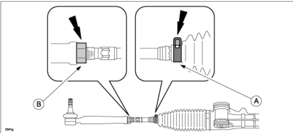
10. Rotate the tie-rod to adjust the steering wheel center. Refer to the following charts for rotating direction.
