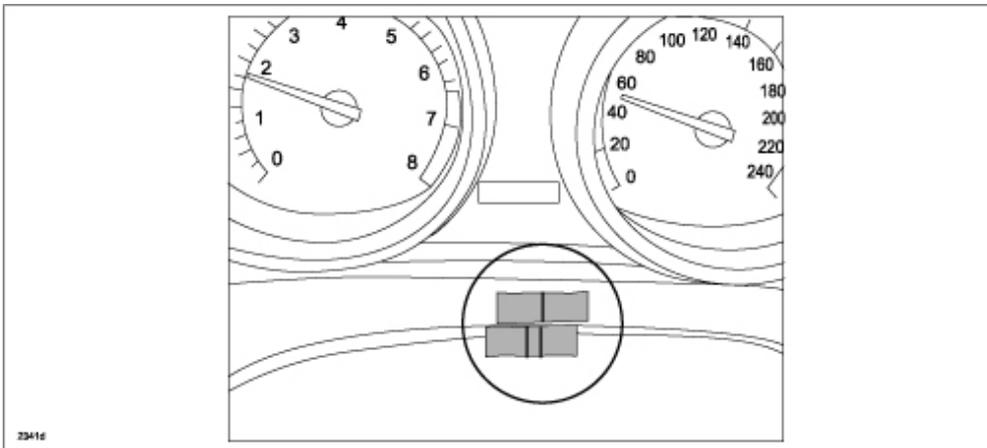
7. Measure the distance between the two lines. The offset can be approximately calculated using  $1\text{mm} = 1^\circ$  of offset.
