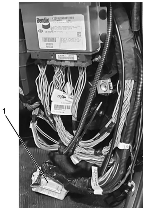
Figure 17. Passenger-side cab 1. 1703M IP-Cowl Interconnect
