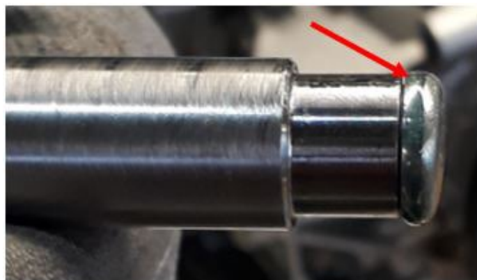
Figure 4. Sealing cap on a drift.
