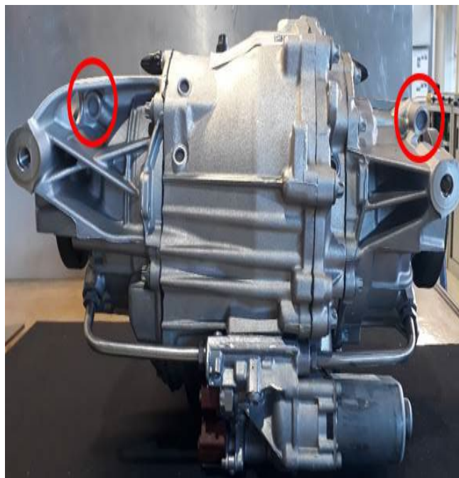
Figure 2. Location of sealing caps on the OD3 differential.
