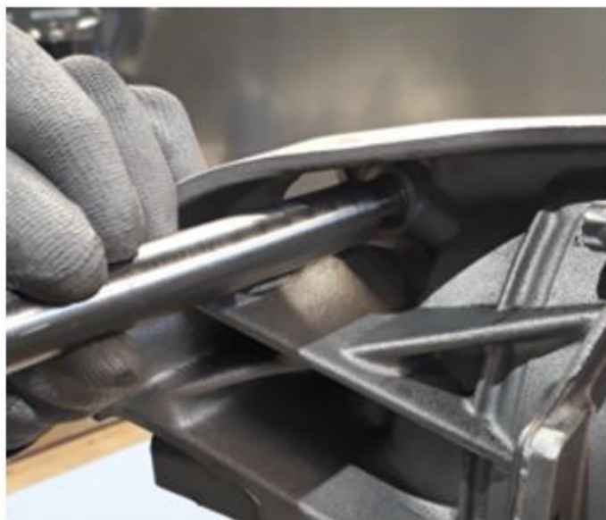
Figure 5. Installing sealing cap
