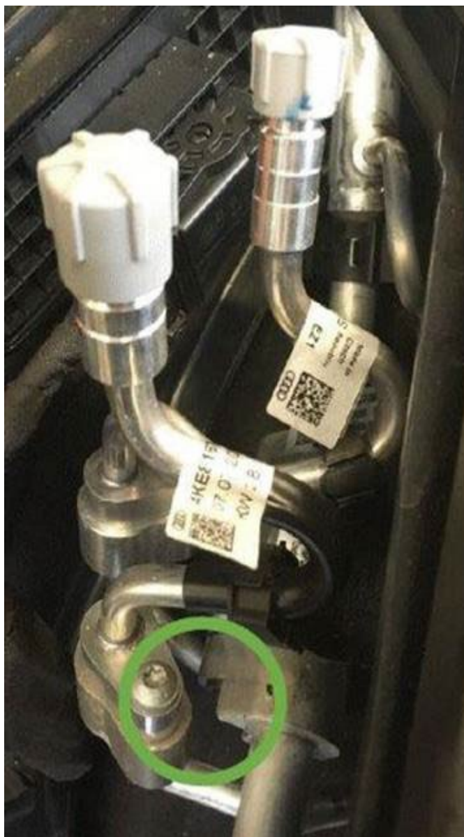
Figure 6. Refrigerant lines retained in a separated position.
