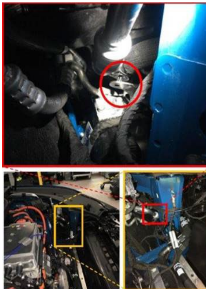
Figure 5. The area in the motor bay where contacting lines are located.
