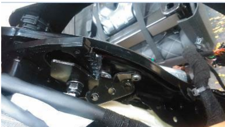
Figure 2. Toothed segment of the seat height adjustment.
