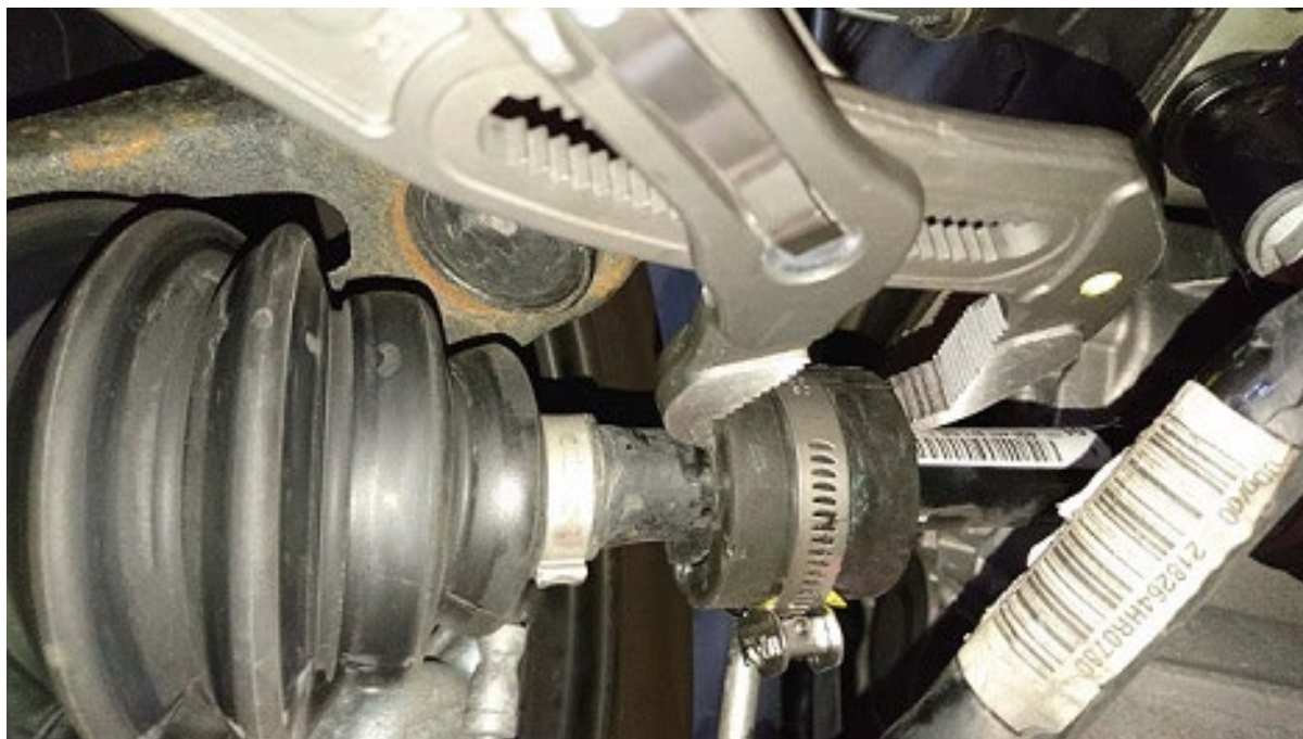
Figure 3. Pressing Roll Pin in Damper
