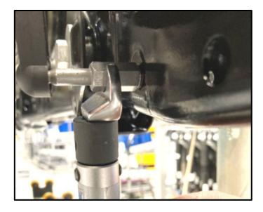
• Re-torque rear level sensor stud.
