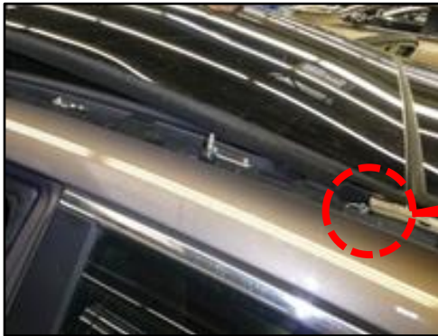
Dust and Dirt Inside Panoramic Sunroof Mechanism
