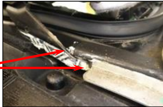
Dust and Dirt Inside Panoramic Sunroof Mechanism
