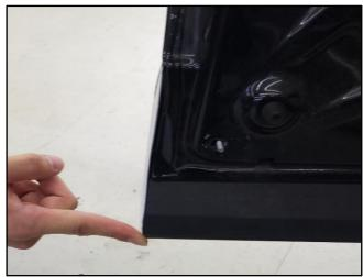
6. If necessary, apply touch up paint to the lower garnish with a touch up paint pen.
