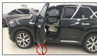
2. Inspect the lower corner where the door garnish and door garnish bracket (A) meet.
