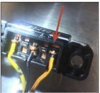
3. Slightly tug the wire from the switch pin a few times. If the wire pulls apart, use a soldering iron to attach the wire to the switch pin.
