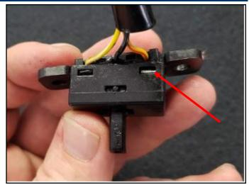
5. If the switch cover comes apart due to broken tabs, replace the switch with a new part.
