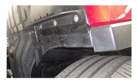
5. Remove the two mounting bolts on the relay box bracket as shown below.
