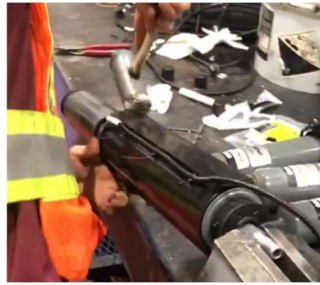
Figure 4: Using Rubber Mallet To Seat Dust Cover on Retaining Ring.
