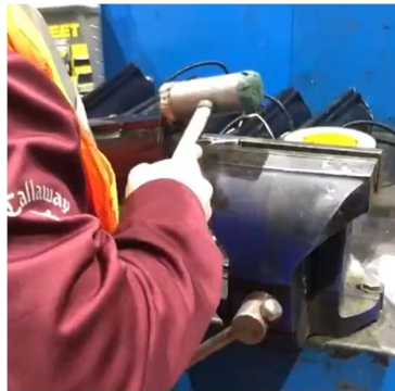
Figure 2: Rubber Mallet Use To Release Dust Cover
