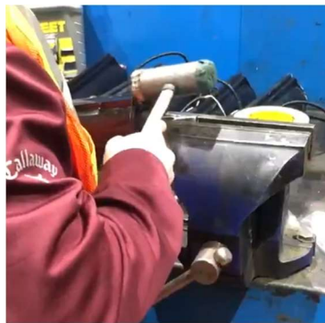
Figure 2: Rubber Mallet Use To Release Dust Cover
