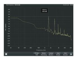
The base frequency shown (1550 Hz) is the noise where the problem is coming from. The other five peaks are all harmonics. This means that if the base frequency is eliminated, the others will go away as well.
