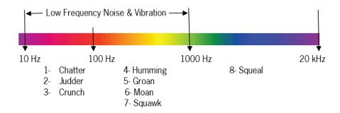
The frequency of the noise will determine what countermeasure to use. Some common design countermeasures are listed below:
