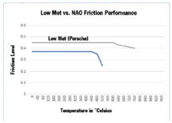
Low met performance characteristics are necessary to maintain the balance of performance in the Porsche vehicle as a whole.
