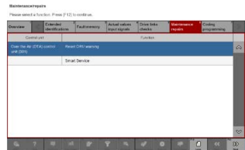
Resetting ORU warning
