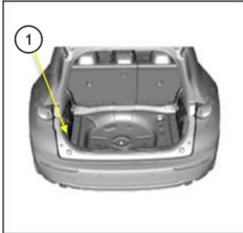
(1) Location of Trunk side insulator
