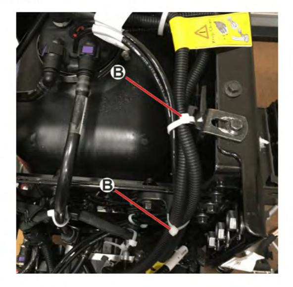
2. Route and tie the UQLS control module routing with the urea harness.
