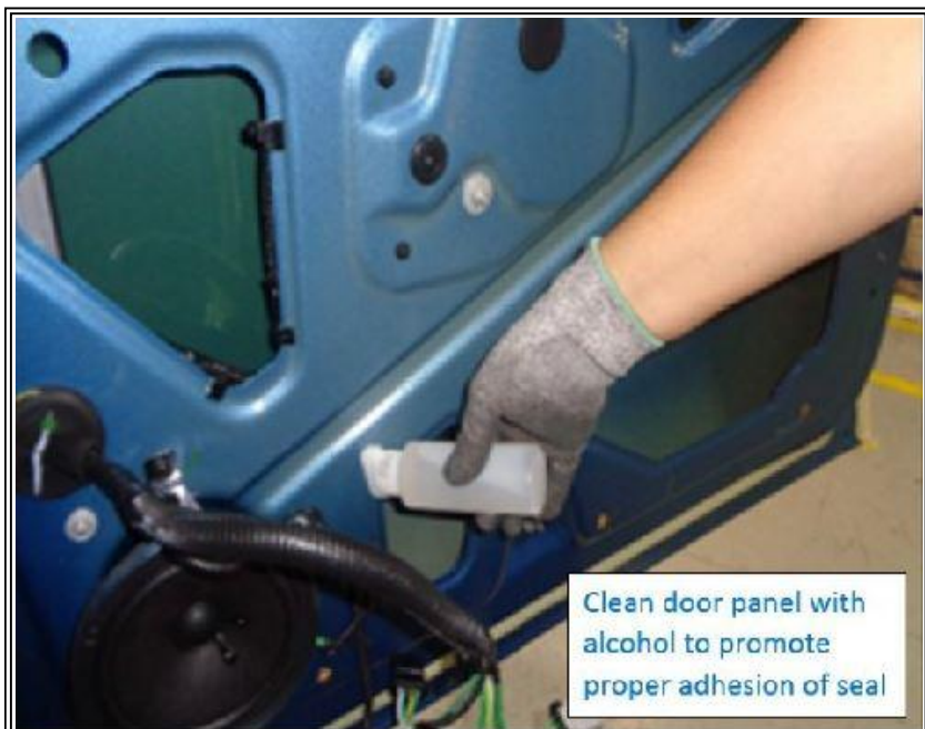
Figure 2: Cleaning the Door Panel of Old Residue
