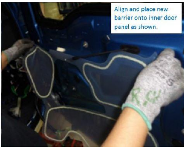
Figure 4: Plastic Vapor Barrier aligned and in place.
