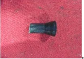
3. Remove the left body mount in front of the rear wheel. Refer to *Body Mount Upper and Lower Cushion Replacement* in SI. There is a rubber cone shaped sleeve in this mount, it can be discarded, it is an assembly aid at the plant.
