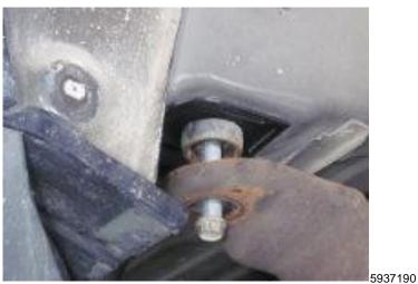
6. Install a suitable nut on the body bolt approximately 25mm (1.0 in.) from the bolt tip. As an alternative, a small section of pipe and a washer can be used as shown in the graphic.
