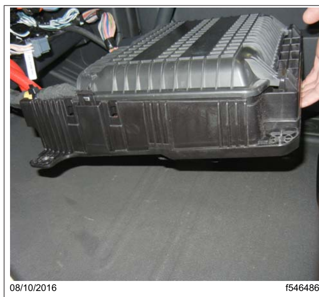
Fig. 14, Lowering the VPDM to the Cab Floor
