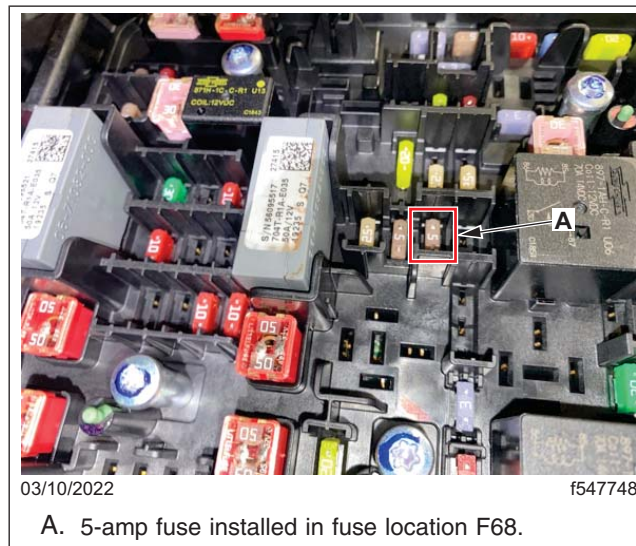
Fig. 12, Fuse Location F68 in the VPDM
