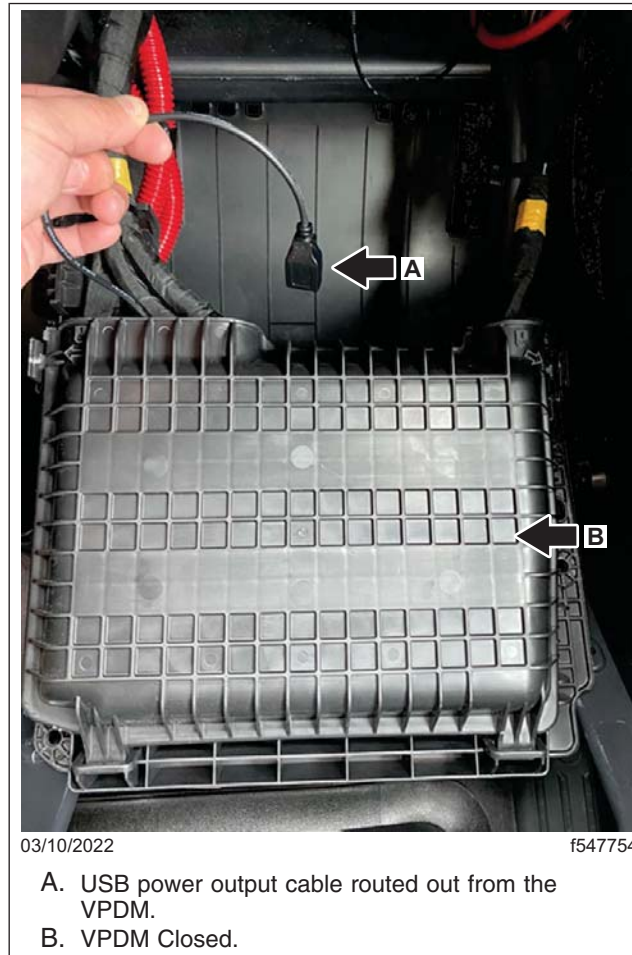
Fig. 20, USB Power Output Cable Routed Out from the VPDM
