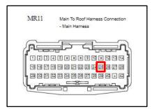
Cut the "red" colored wire 2" inches from the main harness connector and splice the connector end of the "red" wire (5-7mm) where shown.
