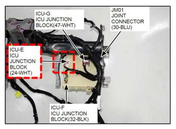
Using a pick tool, pull up on the secondary locking tab to unlock the white junction block wire Pins. <u>Note</u>: Two (2) pull inserts shown.
