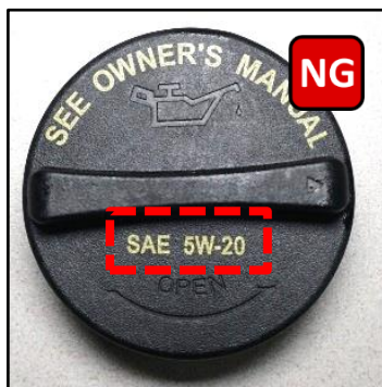
Incorrect Oil Filler Cap (SAE 5W-20)
