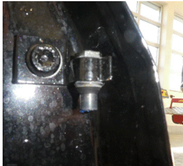
Figure 5. Door hinge pin on door.
