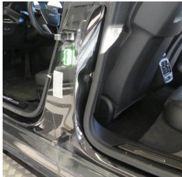
Figure 3. The rear door removed from the vehicle.
