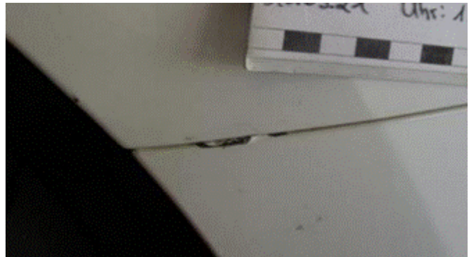
Figure 4. Advanced paint peel.
