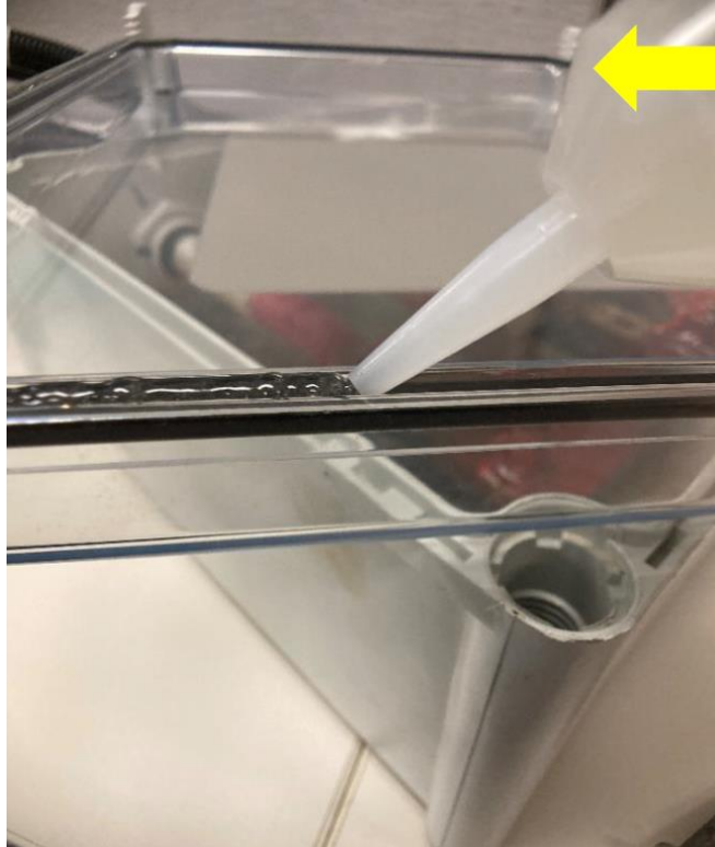
Figure 12: Application of NyoGel on Cover Seal
