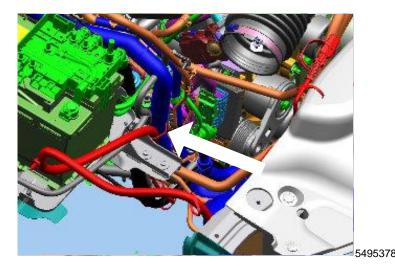
13. Route the power cord (shown in red) as shown and secure to the surge tank hose (blue) with a wire tie.
