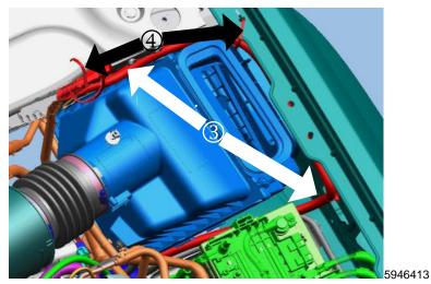
Push pin attachments (3), wire tie attachments (4).
