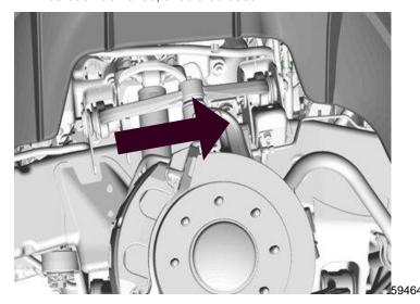
10. Slide the new power cord forward in the vehicle, toward the coolant heater element. Place the power cord connector near the coolant heater element. DO NOT CONNECT the power cord to the heater element at this time, it will be connected after the cooling system pressure test.
