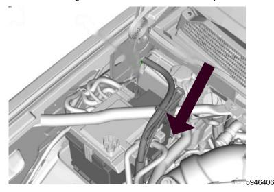
• Start lowering the cord inboard of the battery toward the front of dash.
