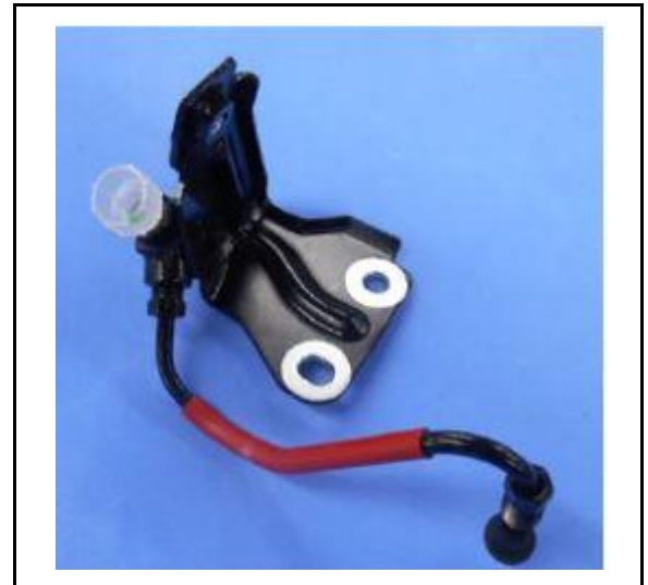
Figure 26. Brake Actuator Tube No. 3 and Brake Actuator Way in the Form of Assembly
