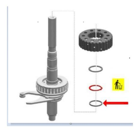
Remove the existing shim, measure it and then replace it with the next smaller shim available. Example shim removed is 4.8 mm then a 4.6 mm should be reinstalled.
