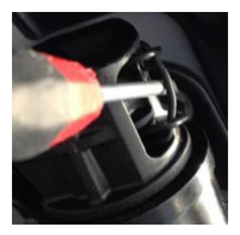
Pull the ball socket off the ball completely.
