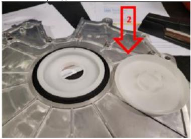
Note: The inner piece is an installation tool designed to be a substitute for the EN52466-2 installation tool. It fits over the bevel on the end of the crankshaft to facilitate installation. Be extremely mindful that the inner lip of the seal slides over the rear of the crankshaft without rolling or a repeat oil leak will occur. The protector/installer has a snug fit to the pilot of the crankshaft.
