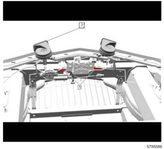
3.1. Remove the left horn (2). Refer to *Horn Replacement* in the Service Manual.
