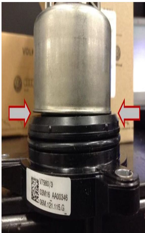
Figure 1. Gap between chamber and seal.
