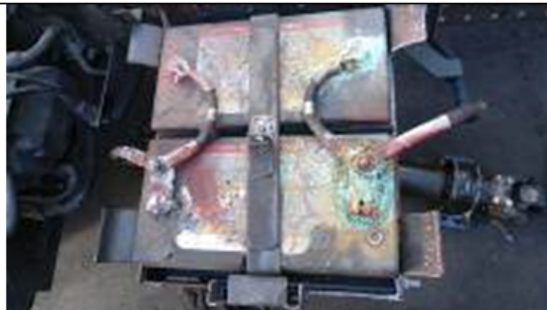
Figure 1 – Example of Water Damage to Battery
