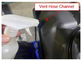
**6.** Spray soapy water on the vent hose nipple of the DEF sending unit and install the vent hose on the DEF sending unit. Ensure that the DEF tank vent hose is fully seated on the hose nipple and is inserted in the channel on the side of the DEF tank as shown in the picture below.
