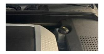
2. Remove the original brake fluid reservoir cap. Replace it with the new one.
