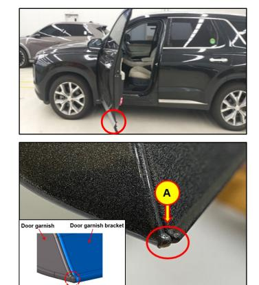
3. Using a razor blade, cut the door garnish (B) along the lower garnish line.
