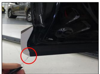
7. Use a heat gun to apply heat in a sweeping motion for approximately 1-2 minutes to assist with drying the touch up paint.
